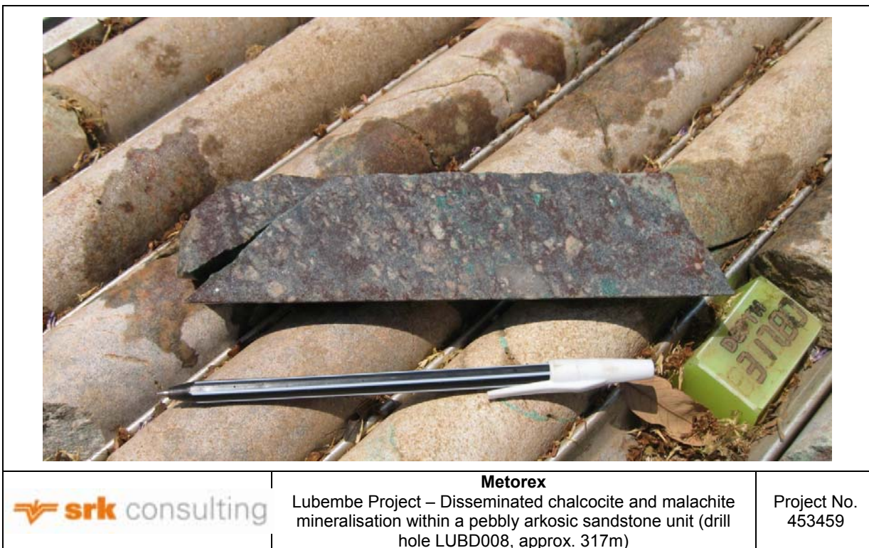
Figure 7.6: Lubembe Project – Disseminated chalcocite and malachite mineralisation within a pebbly arkosic sandstone unit (drill hole LUBD008, approximately 317m) (source: Metorex)
