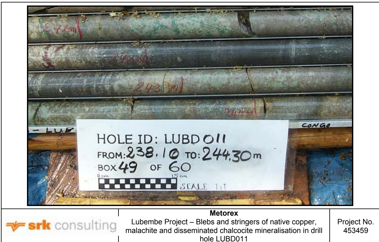
Figure 7.5: Lubembe Project – Blebs and stringers of native copper, malachite and disseminated chalcocite mineralisation in drill hole LUBD011 (source: Metorex)
